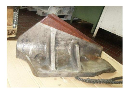
III. 2: GS16MN5N-moldings after de-rusting with ASA Bio-Derosta® L-3
